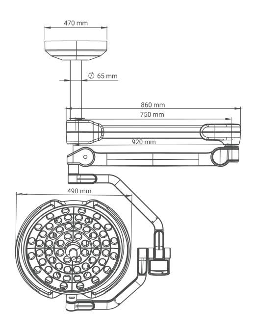
$\bullet \ \ \text{Note:} \ \pm \ 25 \ \text{mm} \ \text{tolerance is given for metric measurements and} \ \pm \ 5^{\circ} \ \text{tolerance is given for angle measurements}.$
